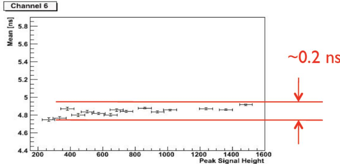
Typical timing resolution achieved  $\sim 1/10$  the sample rate. The PMT shape will drive the ADC sample rate & depth requirements.
