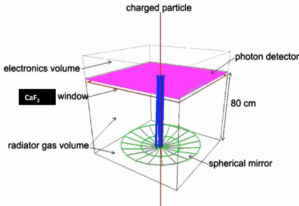
Windowless designs also use  $\text{C}_4\text{F}_{10}$  or  $\text{CF}_4$  as both Cerenkov and amplifier medium.
