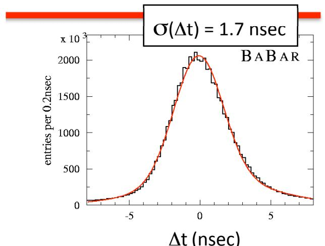
$\Delta t$  also used to determine event time for “self-triggering” of DIRC.
