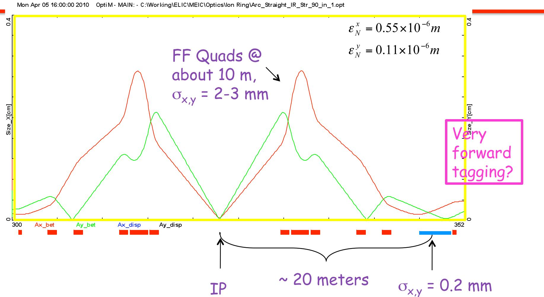
Beam-stay-clear area near IP, before Q1:  $10-12 \sigma \rightarrow 2.5$  cm @ 7 m = 0.2 deg
