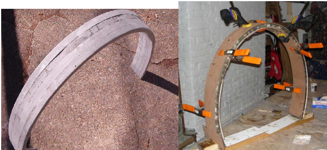
Figures 3.2 & 3.3 Roll bar core & Roll bar clamped in the form
