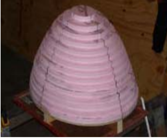
Figures 2.8 & 2.9 Foam plug & Foam plug smoothed with duct tape
