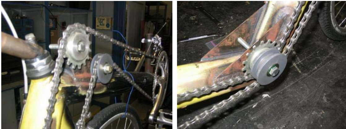
Figure 4.2 & 4.3 Idler wheel supporting chain along the frame of bike
