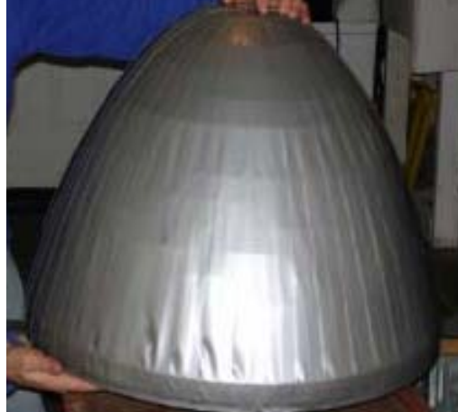
Figures 2.8 & 2.9 Foam plug & Foam plug smoothed with duct tape
