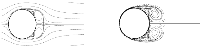
Figure 10 Instantaneous streamlines (left) and vorticity contours (right) of Re = 9500 at t = 4s (Dash line represents the negative vorticity)
