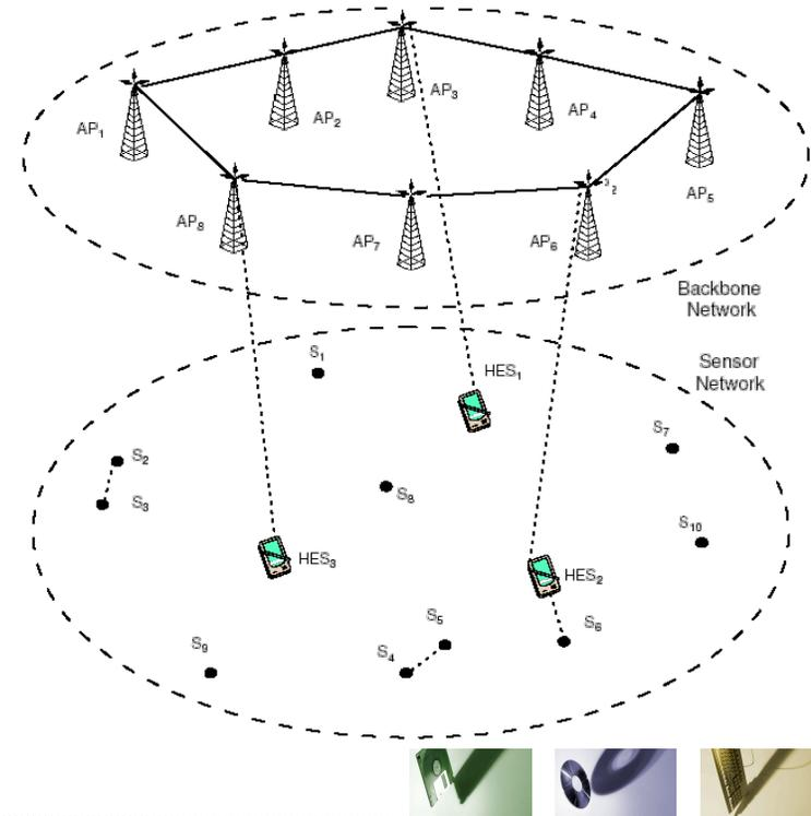
Delay/Fault-Tolerant Mobile Sensor Network (DFT-MSN)
