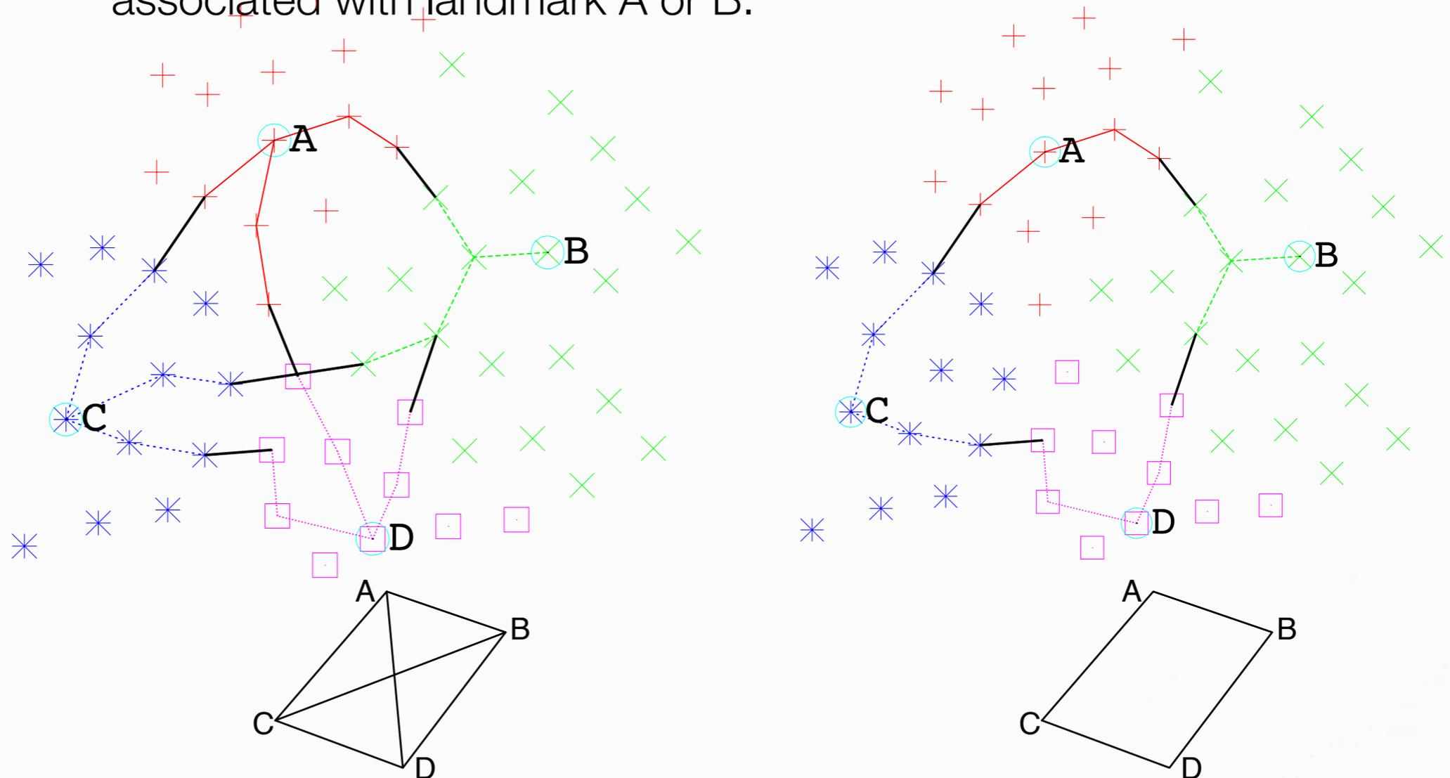
■ Step 4: Construction of Triangular Mesh
