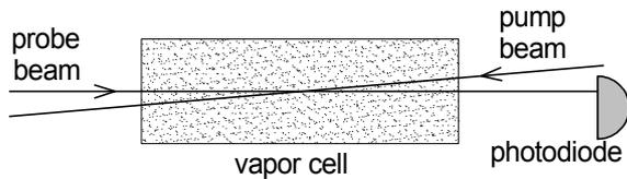
Figure 5: Basic arrangement for saturated absorption spectroscopy.
