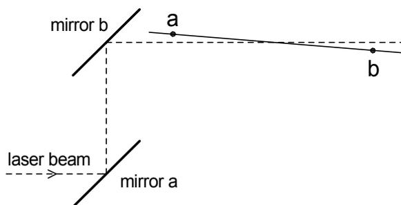
Figure 16: Procedure to align the laser beam (dashed line) along a prescribed line (solid line ab). Pick two reference points a and b and use the first mirror to align the laser to point a and the second mirror to align the laser to point b. Iterate until laser beam is perfectly aligned.
