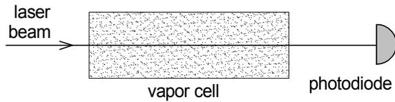
Figure 2: Basic arrangement for ordinary laser absorption spectroscopy.
