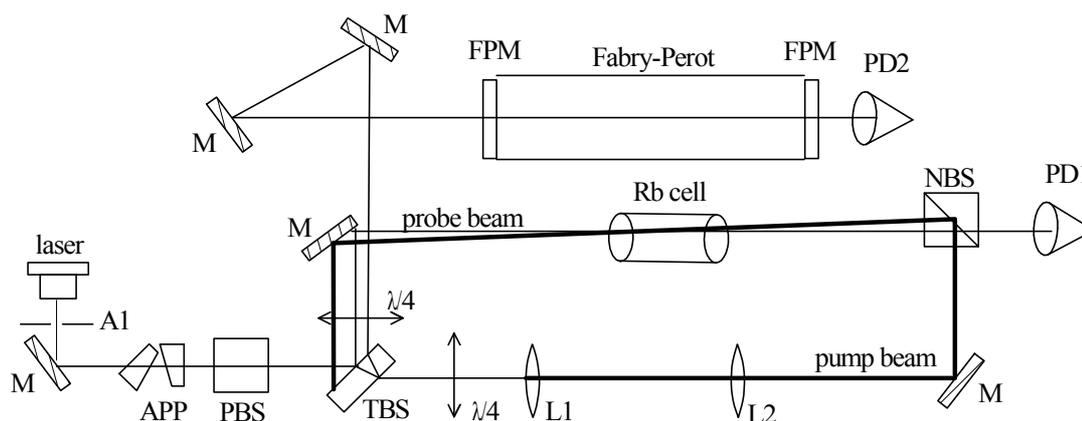
Figure 12: Optical layout of the saturated absorption spectrometer. Key: M mirror; A aperture; APP anamorphic prism pair; PBS polarizing beam splitter; TBS thick beam splitter;  $\lambda/4$  quarter wave plate; L lens; NBS non-polarizing beam splitter; FPM Fabry-Perot mirror PD photodiode detector.
