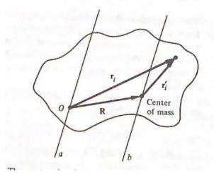
If we look at this image from *Goldstein figure 5.4*, we can see how we have a vector  $\vec{r_i}$  and a center of mass. We can write the vector  $\vec{r_i} = \vec{R} + \vec{r_i}'$ . So the moment of Inertia around an axis a is given by
