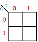
A very handy way to remember the min-term value of each cell is to record that value in the corner of each cell. This will be especially important when you have a numerical canonical list which you wish to map into the graph or you wish to expand an expression into its numerical canonical form. Again, this is the method that you will be REQUIRED to use in any course I teach.
