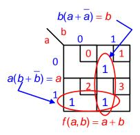
Vertically, it stays in the "1" column, so it can be represented by a '(b)', while horizontally it is in both the 0 and the 1 rows for 'a' and can be represented by a
