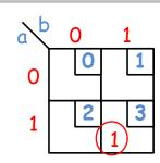
In this case, the MSB (row) heading is a '1' which is an 'a' and the LSB (column) heading is a '1' which is a "b". Therefore, the resulting term is:
