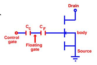
programmer applies a high voltage to the non-floating gate at each bit position where a 0 is to be stored. This causes a breakdown in the insulating material and allows a negative charge to accumulate on the floating gate. When the HIGH voltage is removed, the negative-charge remains. During subsequent read operations, the negative-charge prevents the MOS transistor from turning on when it is selected.
