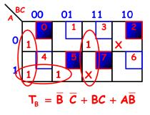
The resulting solution is one of several three term expressions which would describe the required control circuitry for the T input. Note that it isn't very simple and there isn't any way to use illegal states to simplify things.
