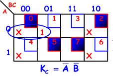
Note that we had to specify replacing it with a 0 or an X since this is a JK which could actually have X's in the columns. Before we update the table we can now simplify  $K_c$ .
