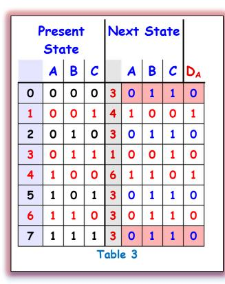
Let's start with the  $D_A$  stage. The  $D_A$ column is created by remembering that the Next State of a D flip-flop will follow whatever value is on the D input when the clock occurs. Thus, the  $D_A$  and  $Q_A$  columns are the same in Table 3.
