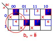
Looking at the new K-map, we note that the included "don'tcares" in states **0** and **5**, provide a simpler control expression. Note that  $\overline{B}$  is nothing more than a wire connecting the **D** input of the A flip-flop (the MSB) to the  $\overline{Q}$  output of the B flip-flop ( $\overline{B}$ ) (the middle bit).
