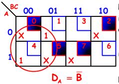
Looking at the K-map, we note that if we include the don't cares in states 0 and 5, we can get a much simpler expression. Note that  $\overline{B}$  is nothing more than a wire connecting the D input of the A flip-flop (the MSB) to the  $\overline{Q}$  output of the B flip-flop (or  $\overline{B}$  )(the middle bit).
