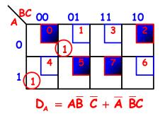
The simplification means that we can get the D flip-flop to act the way we want it to act to create the required sequence if we connect the following control circuitry to it.
