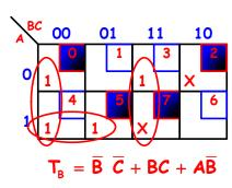
The resulting solution is one of several 3 term expressions which would describe the required control circuitry for the T input. Note that it isn't very simple and there isn't any way to use illegal states to simplify things. Since the specifications allow us to switch to a different flipflop type in order to simply control circuitry, why not replace the T with a D ff?
