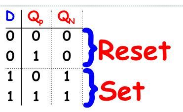
We note that whenever the **D** input is a '0', the output will be 'Reset', while whenever the **D** input is a '1', the output will be 'Set'.
