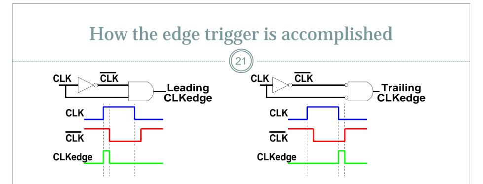
These circuits work by using the fact that there is no such thing as an "ideal" gate. Instead, there exists a delay from the input and the output. The Gate on the far right is a "negative logic" representation of a NOR gate.
