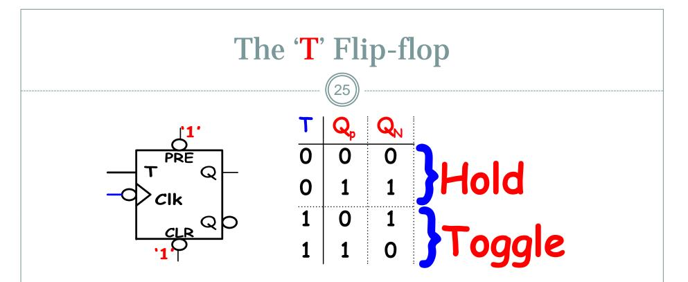
For a 'T' FF, whenever the T input is 'O', the output will be in a 'Hold' condition in which whatever  $Q_p$  is will be held there. Whenever the T input is '1'. the output will be in a "Toggle' condition where if  $Q_p$  is 'O' the output will toggle to a '1' and vice versa.
