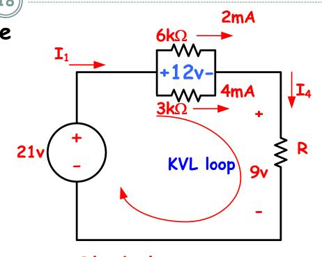
Finally, with the value of  $I_1$ , use Ohm's law to determine the value of R:
