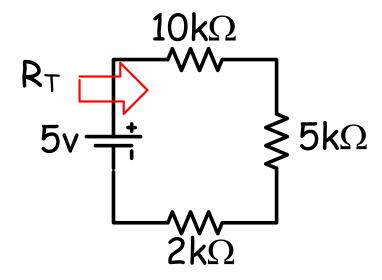
$$R_T = 10k\Omega + 5k\Omega + 2k\Omega = 17k\Omega$$
