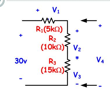
$$V_{4} = \frac{30 (10 k\Omega + 15 k\Omega)}{30 k\Omega}$$
