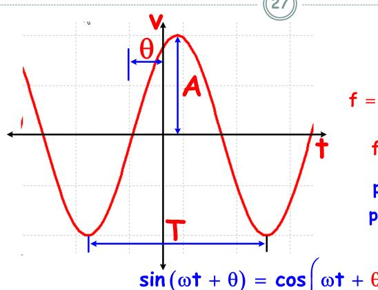
$$f = \frac{\omega}{2\pi} = \frac{1}{T} = \frac{\text{cycles}}{\text{sec}} = \text{hz}$$
