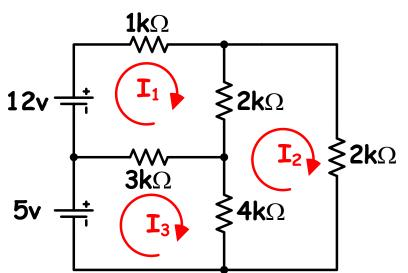
Also note that the sum of the resistors in the I1 loop is 6k just as in the  $2^{2k\Omega}$  the equation. This is another 'idiot' check.
