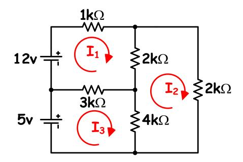
Step 1: It is important that the loop currents be drawn in the clockwise direction
