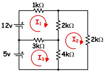
Note that the sign for the current we are working with is + while the signs of both of the others is negative. This is a good 'idiot' check.
