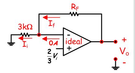
Now we can define this current in terms of  $V_o$ . The "butt" of the arrow is  $V_o$  while voltage at the tip of the arrow is  $(2/3)V_i$ .
