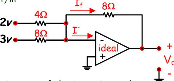
Since the input resistance of the inverting and non-inverting inputs is ideally infinite, the current into those inputs is ideally OA. So the answer is: c) OA
