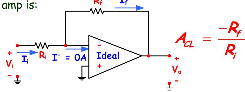
The FE exam uses a (A) for closed-loop gain.
