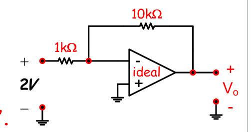
$$V_o = \frac{-R_f}{R_i}V_i = \frac{-10k\Omega}{1k\Omega}(2V) = \boxed{-20V}$$
