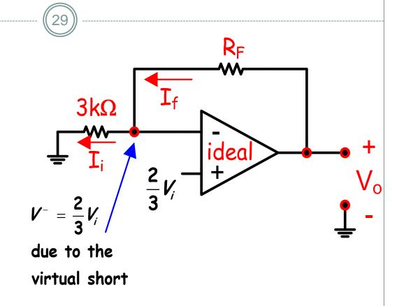
We can now find an equation for  $\mathbf{I}_i$ . The voltage on the "butt" of the current arrow is 2/3  $V_i$  and the voltage at the tip of the current arrow is 0 volts.
