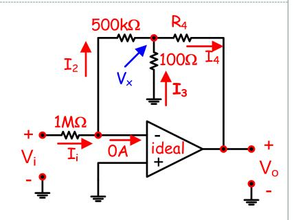
We can use the same technique as before to define  $I_2$  in terms of  $V_x$ . and then equate again to  $I_i$ .
