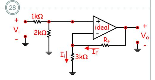
Now that it is flipped over, note that the voltage on the non-inverting terminal is a voltage 'divided'  $V_i$ .
