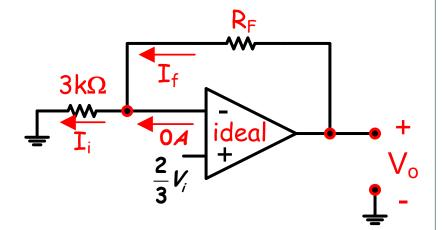
Now, remember that the INFINITE impedance of the Inverting and non-inverting terminals means that the current out of those terminals is "assumed" to be zero. Using this and KCL (above) we find that the feed back current,  $\mathbf{I}_f$  is equal to  $\mathbf{I}_i$ .
