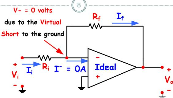
With the addition of two resistors and a ground on the non-inverting terminal we get an "inverting" op-amp. Note that since the non-inverting terminal is grounded the voltage on the "inverting" terminal is also grounded due to the "Virtual" short.
