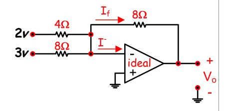
The circuit is an op-amp "summing circuit" or a "Linear Combination Circuit".
