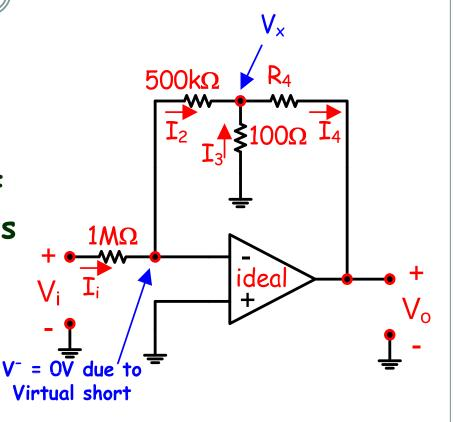
$$I_i = \frac{V_i - Ov}{1M\Omega} = \frac{V_i}{1M\Omega}$$
