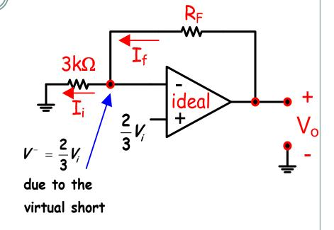
$$I_i = \frac{V^- - 0}{3k\Omega} = \frac{V^-}{3k\Omega} = \frac{\frac{2}{3}V_i}{3k\Omega}$$
