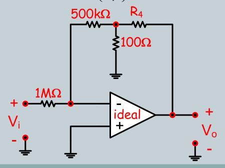
Note that the inverting terminal voltage is 0 volts due to virtual short which exists between it and the non-inverting terminal.
