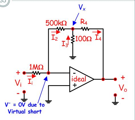
We can now find an equation for the current  $I_i$ . Note that the voltage at the "butt" of the arrow is  $+V_i$  and the voltage at the tip of the arrow is 0v. We use this voltage difference and Ohms law to find an equation for  $I_i$ .
