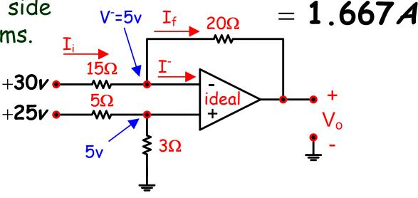
Now we note that since the current into the inverting terminal is zero,  $I_f = 1.667A$  by KCL.
