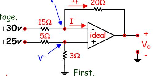
the 5v in the equation is the voltage on the non-inverting leg "voltage divided" between the 5 and the 3 ohm resistors to give us V<sup>+</sup>.
