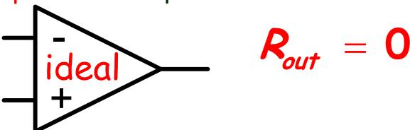
This assumption allows us to make the further assumption that  $V_{\text{out}}$  is independent of the load. This means that it can not be loaded down.
