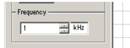
Each cycle will cause one row to be placed on the output ports. You can set the frequency of the waveform in this section. If you are using any of the settings except for "**Step**", you will have to set in your desired frequency in the frequency section. The clock output is called "**Data Ready**." It is the "**R**" output on the device.
