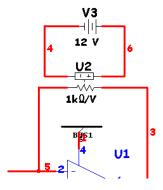
The value of the battery isn't important since you will be sweeping it over a set of values in the DC sweep. In it's present configuration the resistor would be a 12k resistor. Care must be taken in the sweep to keep in mind that the value of the resistor ratio is 1k ohm/v. Feel free to change it to 1 ohm/v if that helps with the values you need to sweep.
