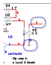
In this case the output node would be Node 9. Note the requirement that the voltage side MUST be grounded. This can also be setup with a resistor on the output stage. This output stage again must be grounded just as it was earlier in the tutorial!
