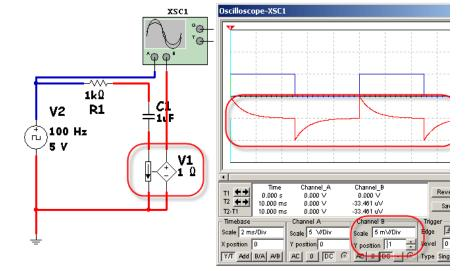
(Note that the output stage of the ICVS is referenced to ground)!!!!
