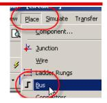
BUS2 Once selected you can draw the bus. <u>It does not have to be a straight</u> <u>line</u>. It can be as long as you want and it can go around corners. Once the bus is drawn a window will pop up with a default bus name. If there are no other bus' on the circuit or if you want to have a new bus with independent connections you can accept the default name.
